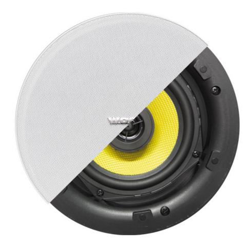
Designed for commercial audio applications, this ceiling loudspeaker has a transducer made of Kevlar, obtaining a high performance in speech intelligibility and musical clarity. Its power selector makes it adapt to high impedance installations (with several positions depending on the model), and low impedance. The loudspeaker body is made of ABS plastic and its metal grill, fixed with magnets, covers almost the entire loudspeaker, making it a discreet element in any installation.
