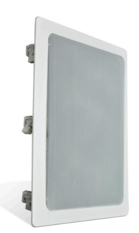
RCS 003 is a 3-way ceiling loudspeaker composed of an 8" woofer, a 2.5" woofer and a 1 "tweeter, which can work in low impedance installations supporting a power of 50 W @ 8 Ohm, and in installations of 70/100 volt line, having a select number of powers (30/20/10 W). Unlike other ceiling loudspeakers, RCS 003 has a square shape, offering an alternative to installers and designers. All range roof is made of ABS plastic and has a metal grill.
