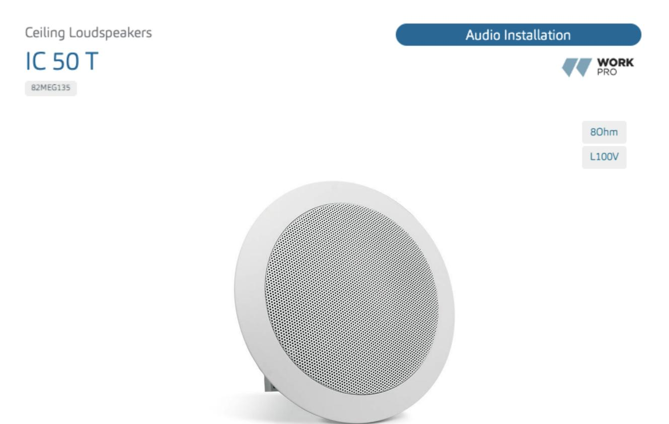
IC 50 T is a ceiling loudspeaker composed of a 5" woofer, which can work in low impedance installations supporting a power of 6 W @ 8 Ohm, and in 100 volt line installations, having a power selector for this. (6/3 W).
