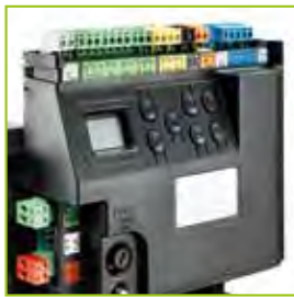
Programming interface and extractable terminal blocks
